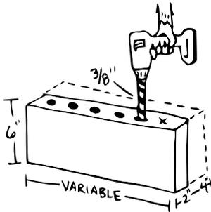
WITH A 3/8" DRILL BIT, DRILL HOLES ON 2" OR 4" FACE OF 2x6" OR 4x6" PIECES OF WOOD. SPACE HOLES 3/8" APART. DRILL HOLES ALL THE WAY THROUGH. SCREW TOGETHER ALL 2x6" BLOCKS. SCREW ON A BACKING BOARD THAT IS TALLER THAN BLOCKS FOR ONE WAY TO HANG OR MOUNT.
